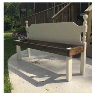
3. The seat of the bench is built of 1x8s and stained walnut. The seat was finished with a more durable polycrylic protective finish. The seat was then attached to the seat base.
